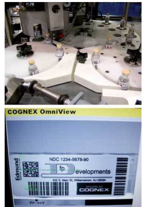
To inspect vial labels, FP Developments has designed a system based on a series of rotary indexing tables (top). After individual vial labels are captured using four cameras, the images are unwrapped, stitched together and OCR and barcode inspection performed (bottom).
